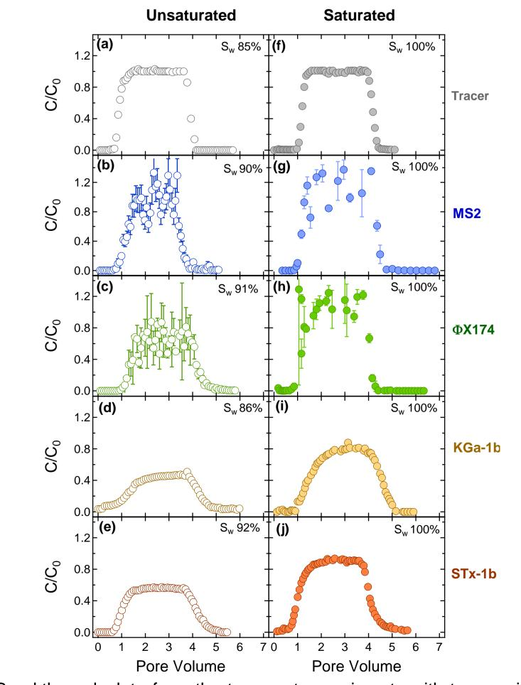
Figure 2. Breakthrough data from the transport experiments with tracer, viruses (MS2 ΦΧ174), and clays (KGa-1b, STx-1b) in unsaturated (a-e: open symbols), and saturated (f-j: filled symbols) columns packed with glass beads.
