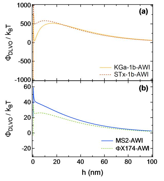
Figure 6. Predicted DLVO energy interactions as a function of separation distance, based on the sphere-plate model for: (a) KGa-1b-AWI, STx-1b-AWI, and (b) MS2-AWI,  $\Phi$ X174-AWI.
