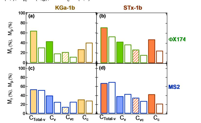
**Figure 5.** Calculated mass recovery values based on C<sub>Total-v</sub>, C<sub>v</sub> and C<sub>c</sub>, and calculated mass produced values based on  $C_{vc}$ , from the cotransport experiments with: (a)  $\Phi X17^2$ and KGa-1b, (b)  $\Phi$ X174 and STx-1b, (c) MS2 and KGa-1b, and (d) MS2 and STx-1b under saturated (filled columns) and unsaturated (open columns) conditions.
