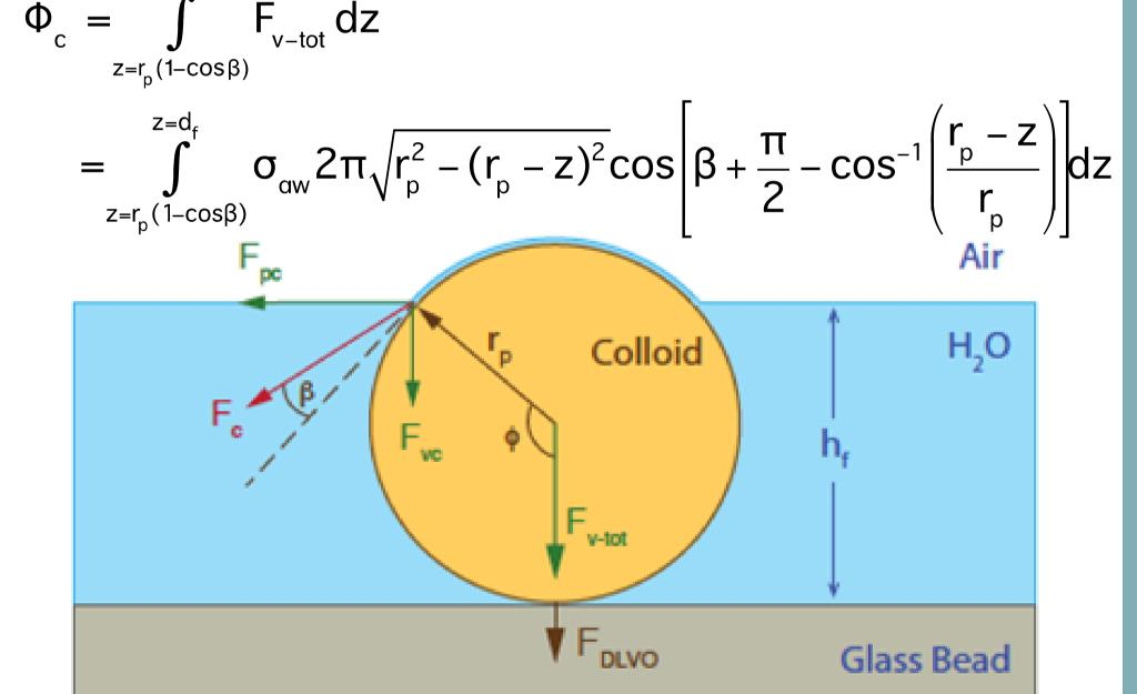
**Figure 1.** Schematic illustration of a colloid with radius r<sub>p</sub>, in contact with a glass bead, trapped in a thin water film with thickness h,
