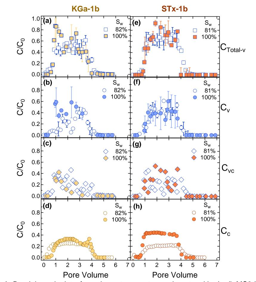
Figure 4. Breakthrough data from the cotransport experiments with: (a-d) MS2-KGa-1b, and (e-h) MS2-STx-1b in saturated (filled symbols), and unsaturated (open symbols) columns packed with glass beads. The concentrations C<sub>Total-v</sub> are presented in (a,e),  $C_v$  in (b,f),  $C_{vc}$  in (c,g), and  $C_c$  in (d,h).
