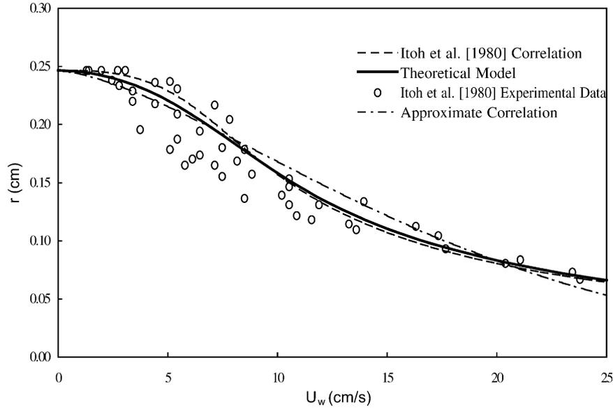
Fig. 6. Graphical comparison of drop radii calculated from the theoretical model, the Itoh et al. [23] correlation, the approximate correlation and the experimental data for benzene drops formed within stream of water flowing perpendicular to the injection nozzle (here  $W = 15$  cm,  $Q_d = 0.0070$  cm<sup>3</sup>/s,  $d = 0.1$  cm,  $\theta = \phi = 0$ ,  $\rho_d = 0.874$  g/cm<sup>3</sup>,  $\rho_w = 0.997$  t/cm<sup>3</sup>).
