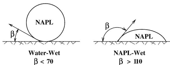
Fig. 2. Schematic illustration of the relative wettability of a NAPL–water–solid system under water-wet and NAPL-wet conditions.
