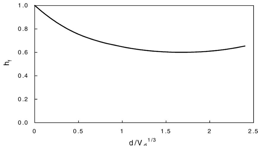
Fig. 5. Harkins' correction factor as a function of the drop volume at the instant of detachment.
