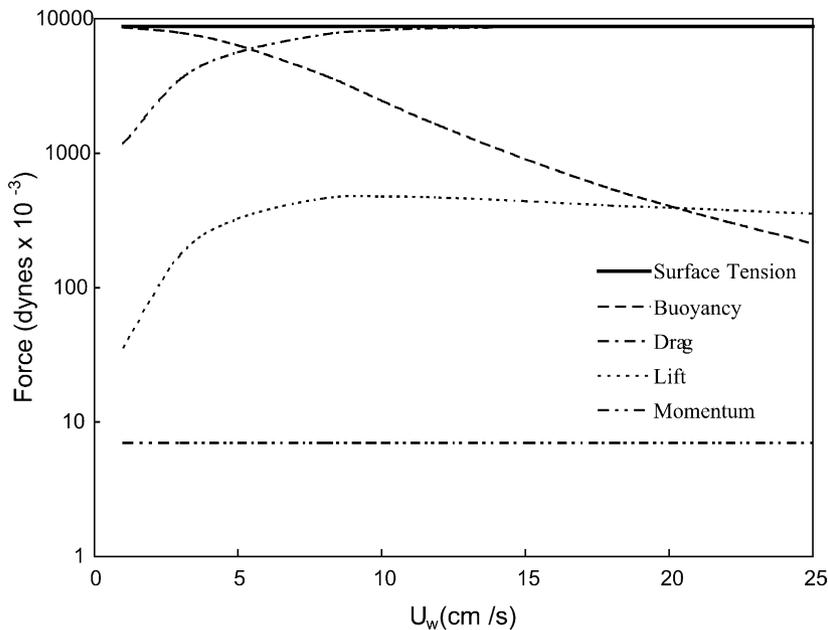
Fig. 7. Graphical comparison of the magnitude of the forces acting on benzene drops at the instant of detachment (here  $Q_d = 0.0070$  cm<sup>3</sup>/s,  $d = 0.1$  cm,  $\theta = \phi = 0$ ,  $\rho_d = 0.874$  g/cm<sup>3</sup>,  $\gamma_{ben} = 28.00$  dyn/cm).
