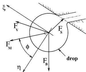
Fig. 4. Schematic illustration of the macroscopic forces acting on a NAPL drop during the drop formation process.
