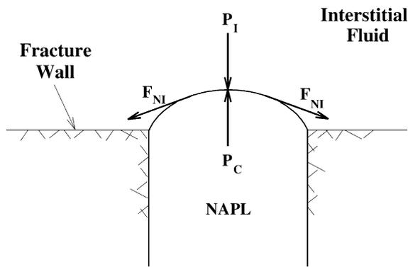
Fig. 1. Schematic illustration of the fluid pressures and surface tension force acting on an exposed NAPL surface as it enters into a fracture ( $P_C$  is the capillary pressure,  $P_I$  is the interstitial fluid pressure and  $F_{NI}$  is the surface tension force at the NAPL/interstitial fluid interface).
