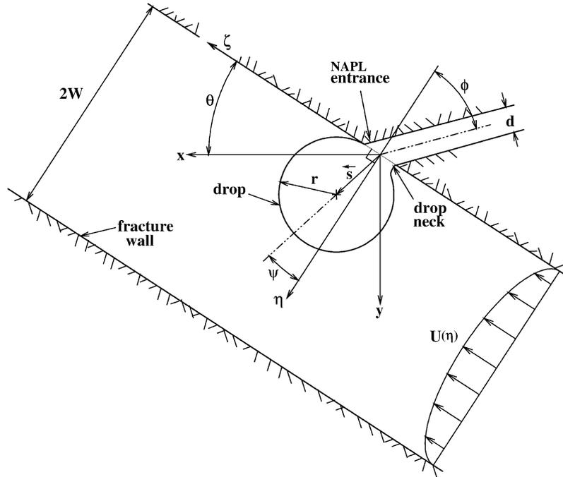
Fig. 3. Schematic illustration of a NAPL drop forming within a uniform, water saturated, two-dimensional fracture.
