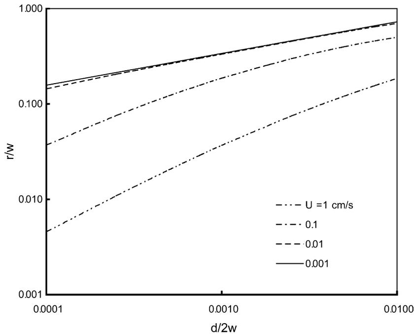
Fig. 8. Graphical comparison of the TCE drop radius generated from the theoretical model for various entrance diameters and interstitial fluid velocities (here  $U_{TCE} = 1.0$  m/year,  $W = 5$  mm,  $\theta = \phi = 0^\circ$ ,  $\rho_d = 1.46$  g/cm<sup>3</sup>,  $\rho_w = 0.997$  g/cm<sup>3</sup>,  $\gamma_{TCE} = 29.6$  dyn/cm,  $\mu_w = 0.8904$  dyn s/cm<sup>2</sup>).
