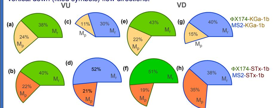
Figure 6. Calculated  $M_r$  values based on  $C_v$  and  $M_p$  values based on  $C_{vc}$  for cotransport of: (a,e) ΦX174 with KGa-1b, (b,f) ΦX174 with STx-1b, (c,g) MS2 with KGa-1b, and (d,h) MS2 with STx-1b under (a-d) vertical upward, and (e-h) vertical downward flow directions.
