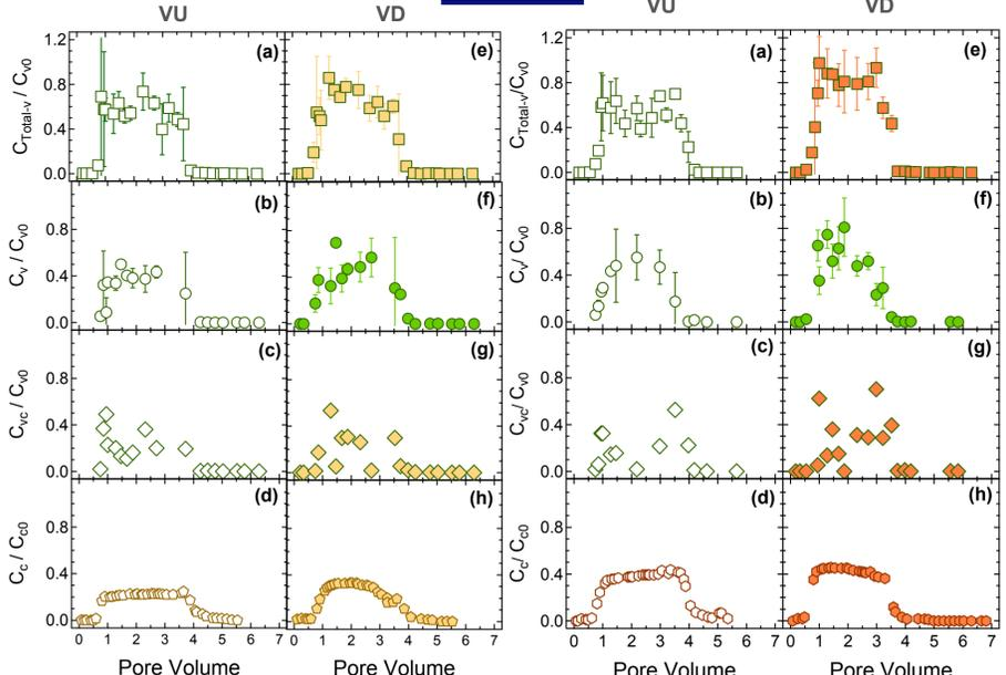
Figures 2-3. Experimental data of  $C_{Total-v}$  (squares),  $C_v$  (circles),  $C_{vc}$  (diamonds), and  $C_c$  (pentagons) for the ΦX174-KGa-1b cotransport (left) and ΦX174-STx-1b cotransport (right) experiments with: (a-d) vertical up (open symbols), and (e-h) vertical down (filled symbols) flow directions.
