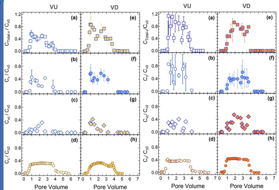
Figures 4-5. Experimental data of  $C_{Total-v}$  (squares),  $C_v$  (circles),  $C_{vc}$  (diamonds), and  $C_c$  (pentagons) for the MS2-KGa-1b cotransport (left) and MS2-STx-1b cotransport (right) experiments with: (a-d) vertical up (open symbols), and (e-h) vertical down (filled symbols) flow directions.
