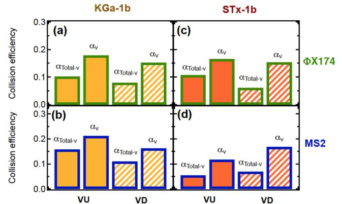
Figure 7. Calculated collision efficiency values,  $\alpha_{Total-v}$ , based on  $C_{Total-v}$ , and  $\alpha_v$  based on  $C_v$ , for cotransport experiments: (a) ΦX174 with KGa-1b, (b) MS2 with KGa-1b, (c) ΦX174 with STx-1b, and (d) MS2 with STx-1b under vertical upward (solid bars) and vertical downward (partially shaded bars) flow directions.
