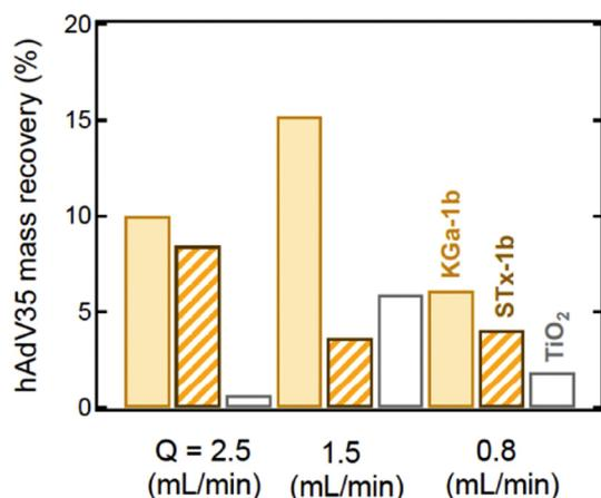
**Fig. 3.** Calculated  $M_r$  values for the hAdV35 cotransport experiments with: KGa-1b (solid bars), STx-1b (cross-shaded bars), and TiO<sub>2</sub> NPs (open bars), for three different flow rates ( $Q = 2.5, 1.5,$  and  $0.8$  mL/min).
