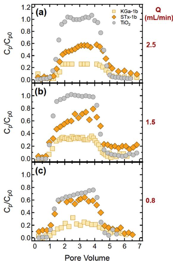
Fig. 1. Experimental effluent normalized concentrations from the transport of KGa-1b (squares), STx-1b (diamonds) and TiO<sub>2</sub> NPs (circles) experiments. Here  $Q$  equal to: (a) 2.5, (b) 1.5, and (c) 0.8 mL/min.
