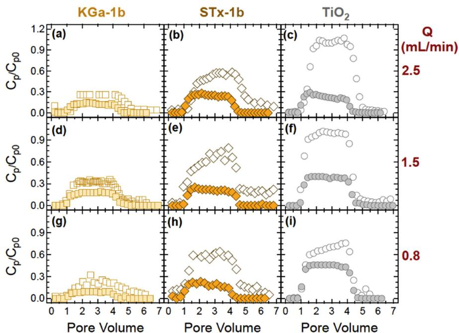
**Fig. 4.** Comparison of effluent normalized concentrations from the transport (open symbols) and cotransport (filled symbols) experiments with: (a, d, g) KGa-1b (squares), (b, e, h) STx-1b (diamonds) and (c, f, i) TiO<sub>2</sub> NPs (circles). Here  $Q$  equals to: (a–c) 2.5, (d–f) 1.5, and (g–i) 0.8 mL/min.
