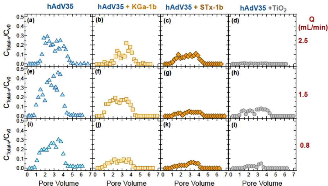
**Fig. 2.** Breakthrough data from the hAdV35 transport experiments (a, e, i) (Kokkinos et al., 2015), and the hAdV35 cotransport experiments with: (b, f, j) KGa-1b, (c, g, k) STx-1b, and (d, h, l) TiO<sub>2</sub> NPs. Here Q equals to: (a–d) 2.5, (e–h) 1.5, and (i–l) 0.8 mL/min.
