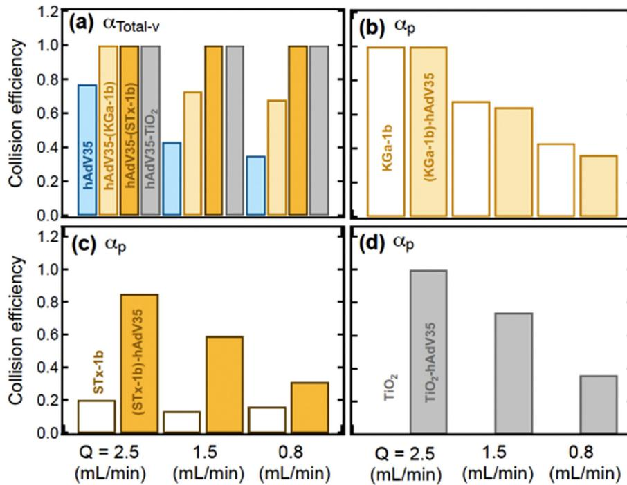
**Fig. 5.** Comparison of: (a)  $\alpha_{\text{Total-v}}$  for hAdV35, (b)  $\alpha_p$  for KGa-1b, (c)  $\alpha_p$  for STx-1b, and (d)  $\alpha_p$  for TiO<sub>2</sub> NPs for transport (open bars) and cotransport (solid bars) experimental data at three different Q values (Q = 2.5, 1.5, and 0.8 mL/min).
